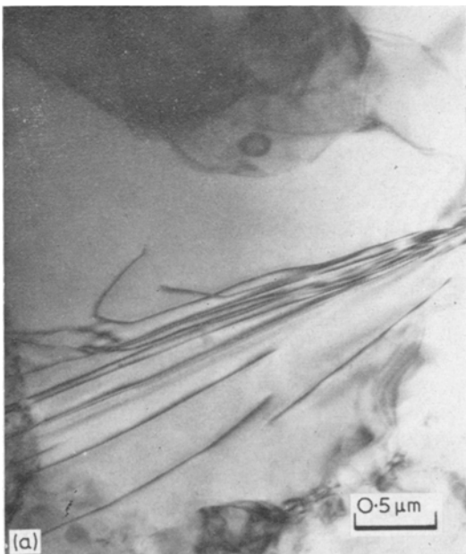
Figure 10 (a) Long dislocations in a large \beta -grain in a reaction sintered specimen. (b) Same area showing one set of dislocations out of contrast, g = [11\bar{2}0] .
