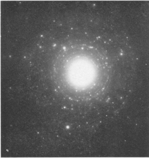
Figure 4 Ring diffraction pattern from fine grained matrix (mainly \alpha -phase).
